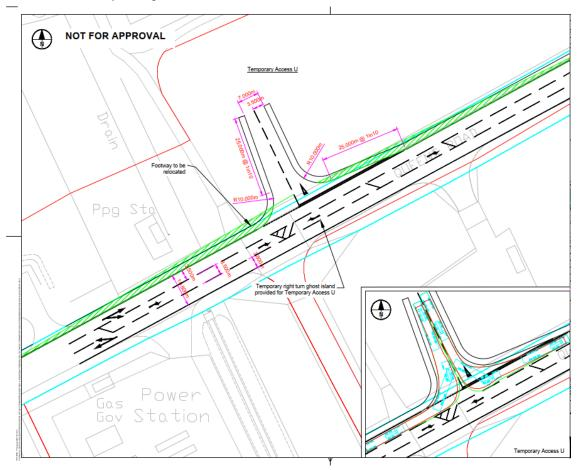
3.1.11 As can be seen in **Plate 11**, Temporary Access U is a right turn ghost island from Kings Road and has been designed to accommodate max legal HGV movements.
