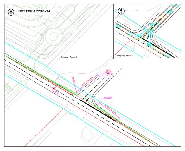
3.1.10 As can be seen in **Plate 10**, Temporary Access P is a simple priority junction from Laporte Road and has been designed to accommodate max legal HGV movements.
