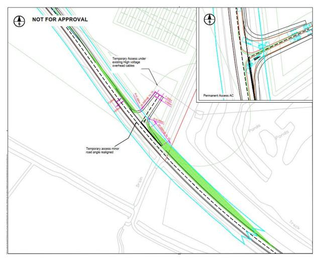
3.1.6 As can be seen in **Plate 7**, Temporary Access AC is a simple priority junction from the A1173 and has been designed to accommodate max legal HGV movements.
