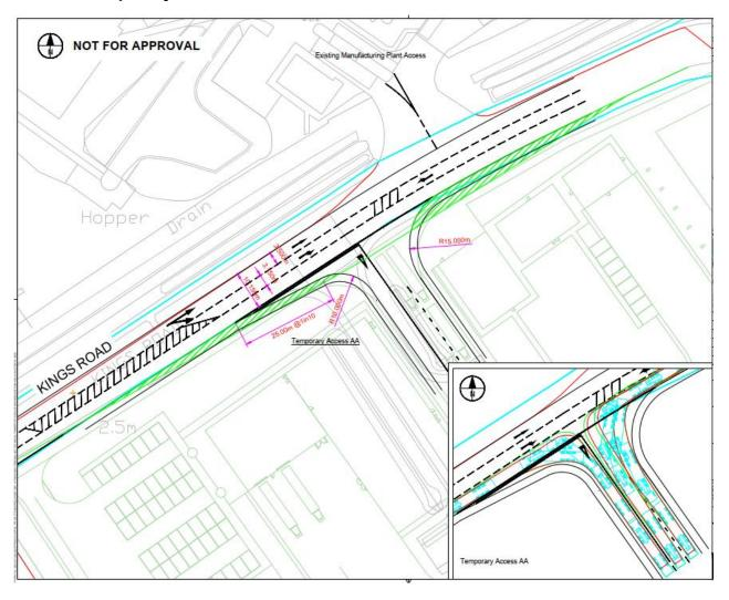
3.1.4 As can be seen in **Plate 5**, Temporary Access AA is a right turn ghost island from Kings Road and has been designed to accommodate max legal HGV movements.
