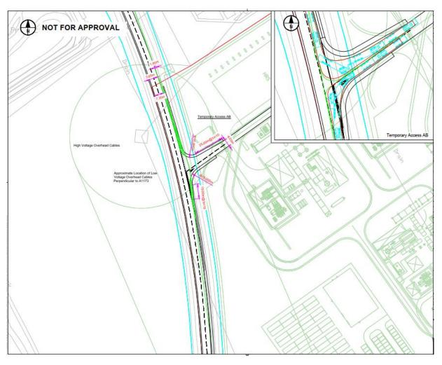
3.1.5 As can be seen in **Plate 6**, Temporary Access AB is a simple priority junction from the A1173 and has been designed to accommodate max legal HGV movements.
